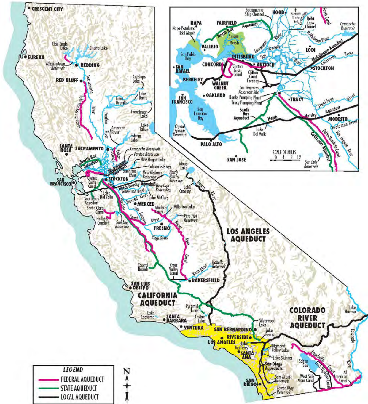
Figure 4-3. Major Water Conveyance Facilities in California
