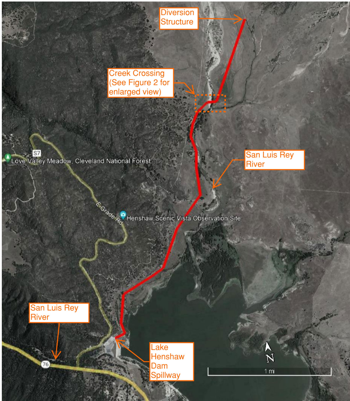
Figure 4-9. Lake Henshaw bypass pipeline preliminary alignment.
