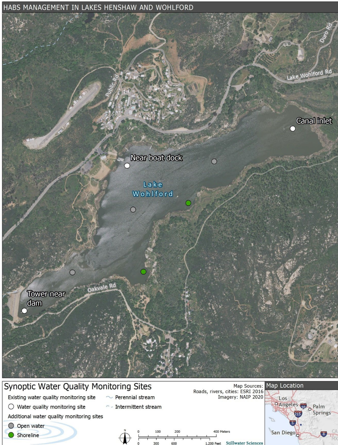
Figure 5-7. Approximate locations of monitoring sites to establish index sites and rapid response monitoring sites in Lake Wohlford. Existing canal inlet, near boat dock, and tower near dam sites (white circles) will be included. One open water site nearest the existing aeration diffuser (orange circle) will also be included.
