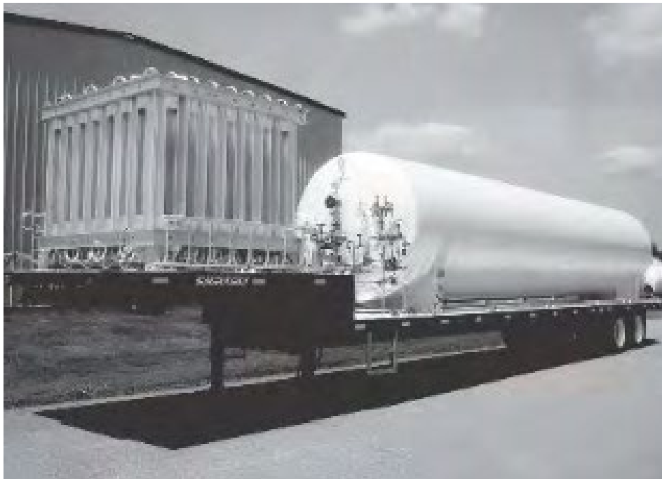
Figure 4-8. Example trailer-mounted LOX and vaporizer—typical configuration.
